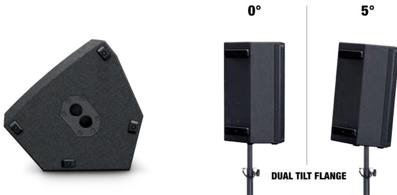
The speakers have a stand flange with a 0° angle socket (rear position) and a socket with a 5° tilt angle (front position). Examples of use: Use the socket with the 0° angle for standing audiences and the socket with the 5° tilt angle for seated audiences.
